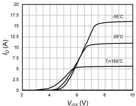
Figure 5. Transfer Characteristics
