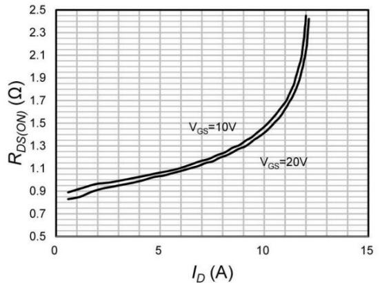
Figure 2. Drain-Source On-State Resistance vs. Drain Current
