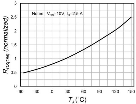
Figure 3. Drain-Source On-State Resistance (Normalized)
