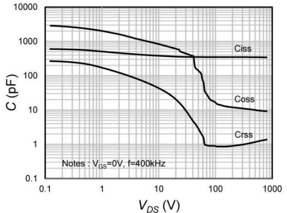
Figure 8. Capacitance Characteristics
