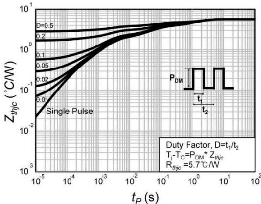
Figure 13. Transient thermal impedance
