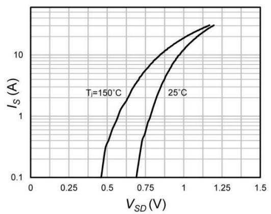
Figure 6. Forward Characteristics Of Reverse Diode
