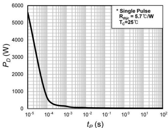
Figure 11. Power Dissipation
