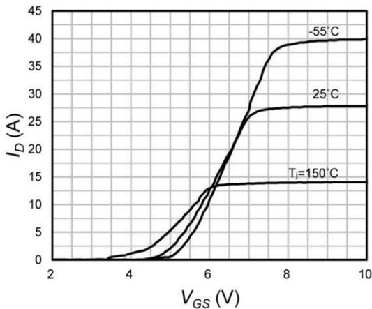
Figure 5. Transfer Characteristics
