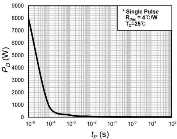
Figure 11. Power Dissipation
