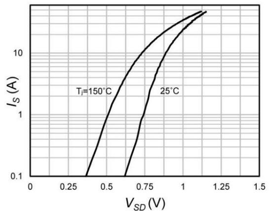
Figure 6. Forward Characteristics Of Reverse Diode
