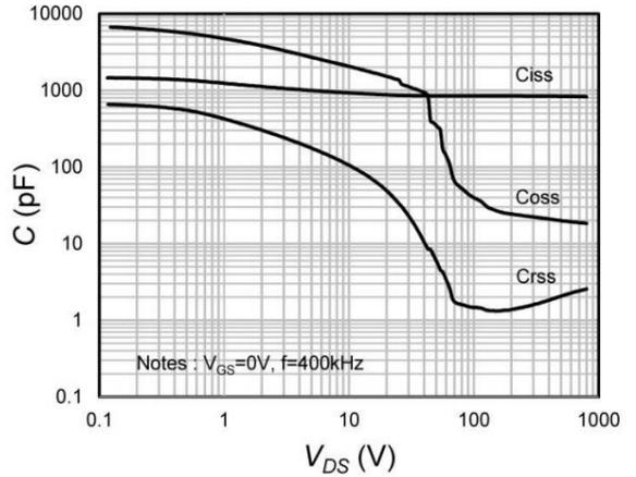
Figure 8. Capacitance Characteristics
