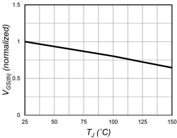
Figure 9.  $V_{GS(th)}$  variation vs. Temperature (Normalized)
